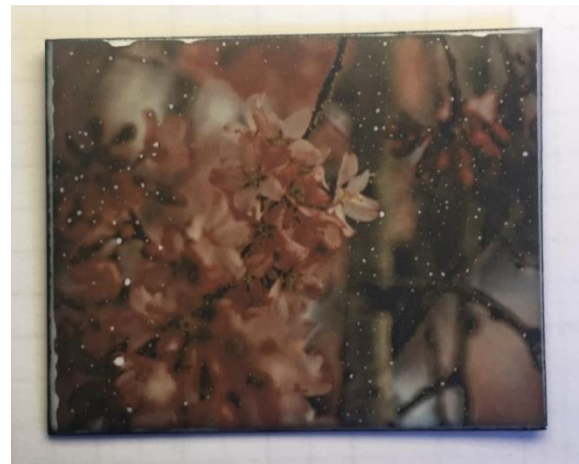
Fig. 12. Color photo decal, fired at 1420° F.
