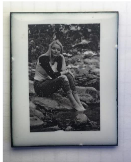
Fig. 10. New firing time for black-and-white photo decals reveals sharper images with minimum water/air marks.
