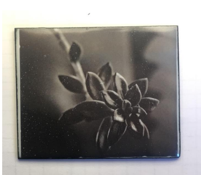
Fig. 9. New firing time for black-and-white photo decals reveals sharper images with minimum water/air marks.
