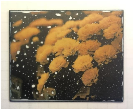
Fig. 11. Color photo decal, fired at 1420° F.
