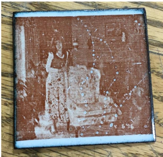
Fig. 5. Single firing at 1450° F with evidence of water/air bubbles.
